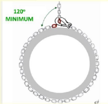
Minimum spreading angle of the cable when the load is tied [16]
