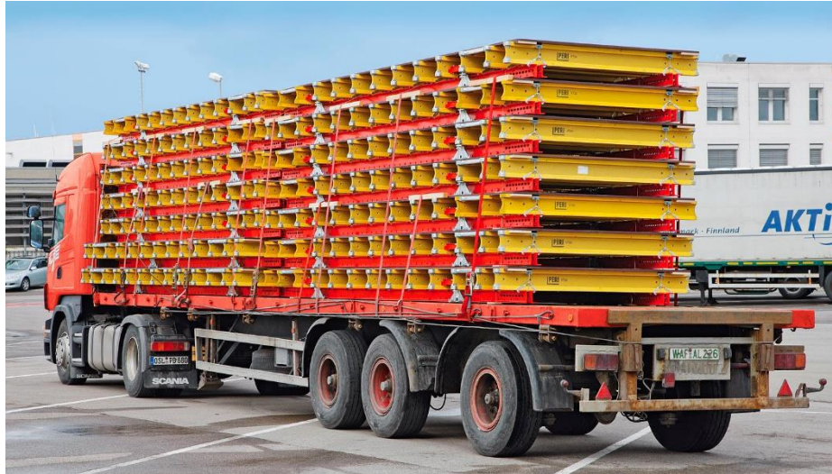
Fig. Transportation of formwork [Source: PERI]
